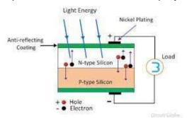
of electrons available, that need lower threshold energy to get excited and break the balance, thus generating electricity. When sunlight falls upon the photodiode, the electrons present in the valence band absorb energy and jump to the conduction band to become free. Some of these electrons are even accelerated through the rectifying junction due to built-in potential, thus ending into the p-type semiconductor material This generates movement
