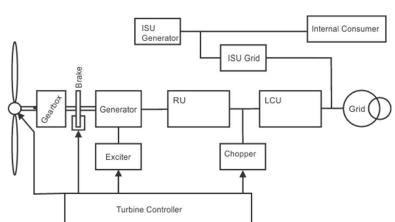
turn use it to turn electrical generators and generate power. Today, most turbines use variable speed generators combined with partial- or full-scale power converter between the turbine generator and the collector system, which generally have more desirable properties for grid interconnection and have Low voltage ride through-capabilities. Modern concepts use either
