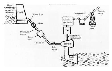
Hydroelectric power plants can include a reservoir (generally created by a dam) to exploit the energy of falling water, or can use the kinetic energy of water as in run-of-the-river hydroelectricity. Dam based power plants provide more dependable generation, as they eliminate the risk of decrease in flow of water with changes in seasons.
